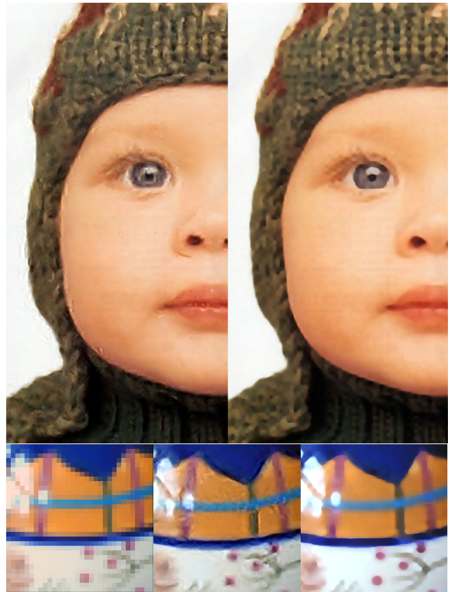
Figure 8: Top to bottom, left to right are: child's face upsampled by a factor of 4 using the Example-Based Super-Resolution, and using our method. Bottom row shows pixels of a teapot, their magnification by a factor of 8 using the Example-Based Super-Resolution, and the result of our method. Both the teapot original image and the images generated by the Examples-Based Super-Resolution are courtesy of William T. Freeman.
